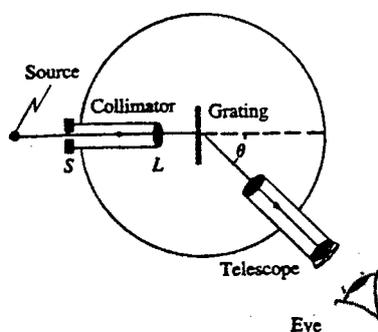
The light from the source passes a collimator. The diffracted ray is observed directly through a telescope. The angle  $\theta$  is shown on the scale of the spectroscope table.
